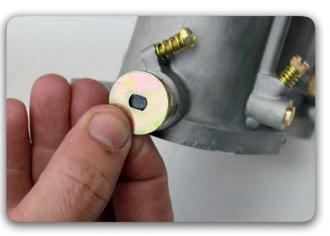
STEP 2 - Install the throttle shaft spacer.
