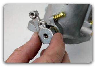
STEP 3 - Thread the "true position" throttle arm onto the throttle shaft. It is not necessary for the throttle arm to touch the spacer. The spacer is only needed to take up the airgap between the carb and the throttle arm.
