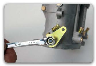
STEP 1 - Using an 11mm Wrench, remove the throttle shaft lock nut and throttle arm.
