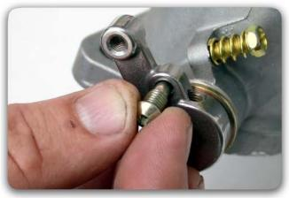
STEP 5 - Install throttle stop into the "true position" throttle arm. Use a small drop of red loctite on threads.
