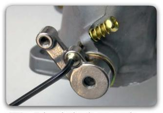
**STEP 6** - Tighten the throttle stop securely using a 7/64" allen wrench.
