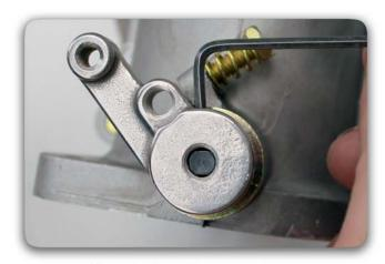
STEP 4 - Align the throttle arm so the set screws line up with the flattened sides of throttle shaft. Tighten the set screws securely using a 3/32" allen wrench.
