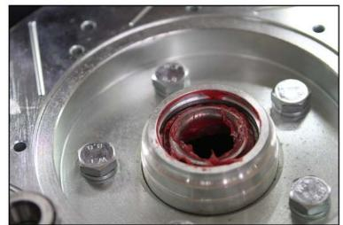
7 - Grease the wheel bearings using Disc Brake wheel bearing grease.
