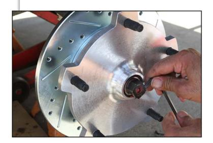
11 - Install the Wide 5 rotor assembly on the spindle, slide the outer wheel bearing into place and install the spindle nut and washer. Adjust bearing free-play and torque per factory specs.
