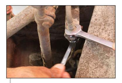
3 - Remove rubber flex brake hose from the hardline, be careful not to round off the hex nut on the original hardline; it is best to use a brake-line wrench for this job. You will also need to remove the spring clip that holds the rubber flex hose in place.
