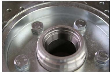
**6** - Install the inner and outer bearing races into the wide 5 hub. Be careful not to pound the races in too far as this will destroy the aluminum hub.
