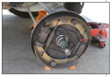
2 - Remove front wheels and brake drums.
