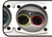
Relocated exhaust quides allow for additional material between the seats, improving head strength and allowing for valve sizes up to 46 x 37.5!
