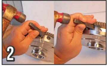
Mark 1st weight ring and flywheel for re-assembly.
