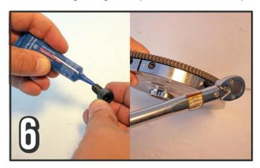
Apply red loctite to all eight mounting bolt threads, and torque to 30 ft-lbs.
