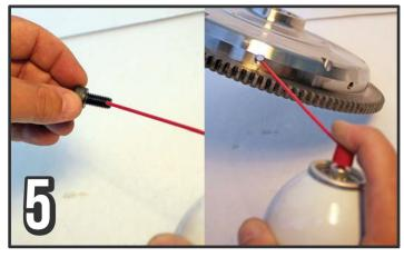
Clean threads on mounting bolts and flywheel with Carb Cleaner or Brake-Clean.
