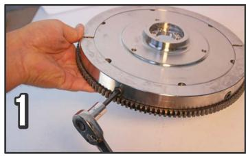
Remove mounting bolts on one weight ring.
