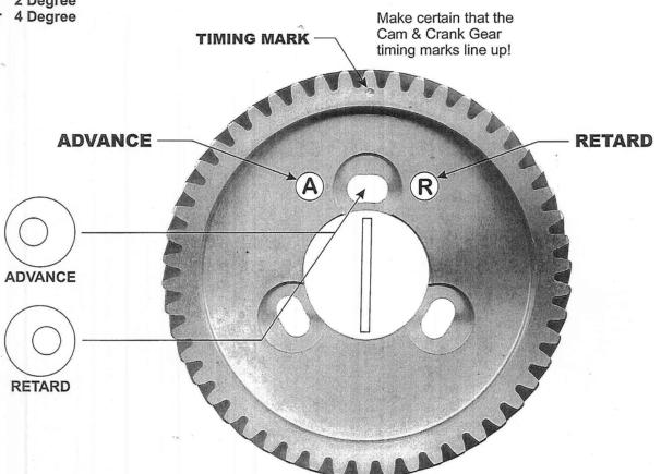
Place the desired degree washers on cam gear followed by the Wave-loc washer and bolt. Torque the bolts to 20 foot pounds.
