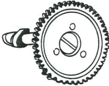
FIGURE 1 Early Cam may be equipped with rivets as shown, or 8mm bolts.
