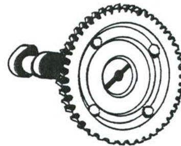
FIGURE 2 Late Cam for use with long shaft Oil Pump.
