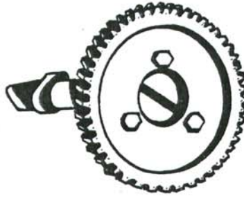
FIGURE 1 Early Cam may be equipped with rivets as shown, or 8mm bolts.
