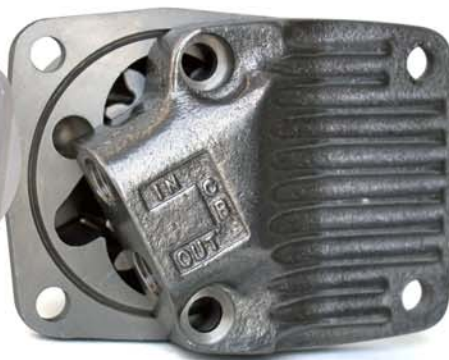
FIGURE 1 Early Cam may be equipped with rivets as shown, or 8mm bolts.
