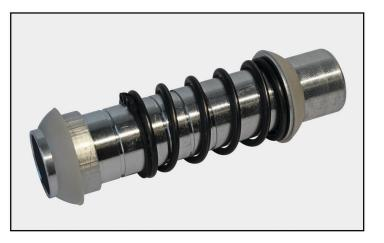
**STEP 3**Add Spring, Washer and Seal to the Inner/Lower Tube.
