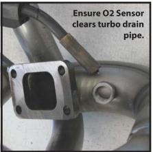
somewhere between the 10 O'clock and 2 O'clock position. Turbo Applications: Weld the O2 sensor bung in the collector. Please refer to the pictures above to see the recommended placement of the O2 sensor.
