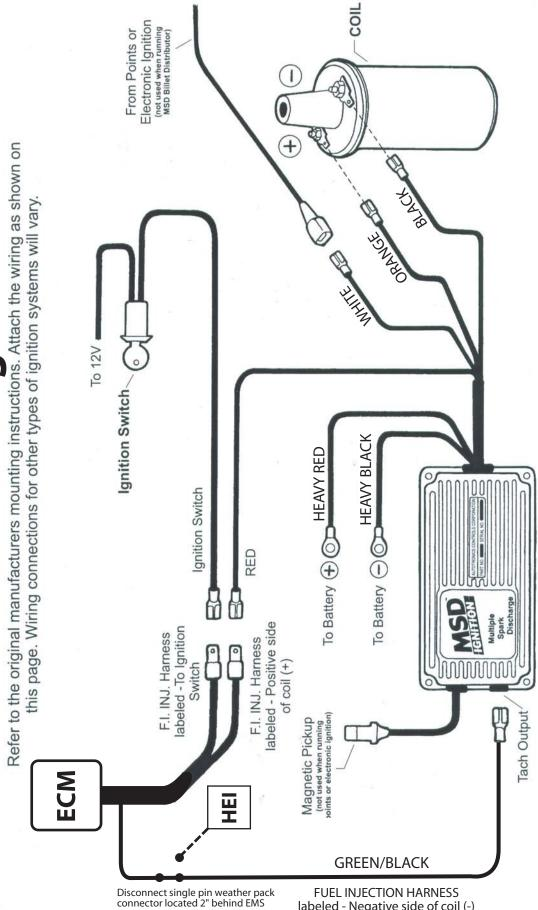
connector. Connect the provided MSD adapter wire to the single pin connector leading to the EMS. Connect other end of MSD adpater to the MSD tach output.
