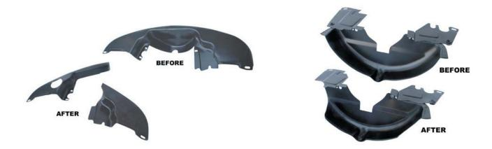
Here you can see some before and after pics of some Engine Sheet Metal that has been modified to run on a Turbo System.
