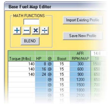
F) Go down the RPM column until you find the RPM where you believe your engine will produce peak torque. Double left click on this cell and type in your peak torque value.
