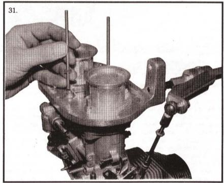
disassembly of the carburetors, minor air flow changes can be effected by opening or closing the air by-pass screws. This procedure is initiated by confirming that all of the air by-pass screws were turned out one half turn from the bottom during
