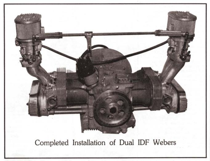
dialing in your duals that helps engines run silky smooth. Adjust the uni-syn gauge to flow and register at the lowest mark on the indicator tower. This reduces the possibility of choking the engine while the uni-syn gauge is in position on top of the barrel. If a barrel shows less air flow than the previous cylinder, increase the air flow by opening up the air by-pass screw. Conversely, air flow can be reduced by closing the by-pass screw. Refer to picture (30).
