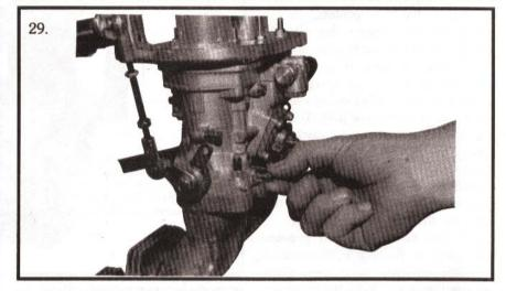
remaining mixture screw, 4, 2 and 1. Refer to picture (29). If repositioning a mixture screw, turning it in, shows no effect on engine operation, it has to be assumed that either a vacuum leak exists on that barrel, the spark
