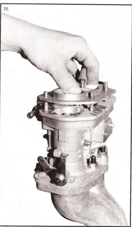
position. So make certain to use the long studs where needed. Now move on over to the other carburetor and repeat the procedure.
