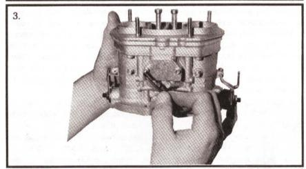
situation. You or the carburetors. Pre-tuning is initiated by setting all of the butterflies at the same opening. This is accomplished by using a .004 steel feeler gauge placed between the butterfly and the side of the carburetor barrel wall. Refer to picture
