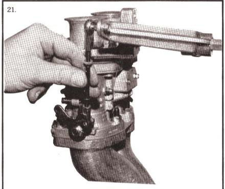
two helper throttle return springs. The helper springs provide a safety factor and should be seriously considered for use on any type of vehicle. The slight amount of increase in throttle pressure will never be noticed.
