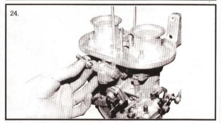
that it works free and returns to idle position. Throttle cables that are too short will prevent the linkage from returning to idle speed. Check the idle speed throttle stops, they should rest against the idle speed screws. All nuts and screws should be snug, fuel lines securely in position and mounted in a location to prevent interference with linkage movement. Tie those new spark plug wires out of the way. Don't let'em get jammed up in your linkage shafts or throttle arms.
