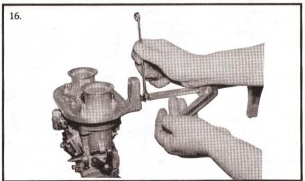
carburetor barrel walls. Once the nut has been removed the locking plate will now come off. The linkage arms should be put on so that they are facing inward towards one another. Refer to picture (17). Now the locking plate can be put back on followed
