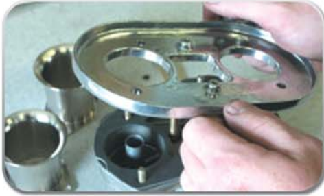
1 - Remove the Air Cleaner from the Carburetor and separate base from Air Cleaner.
