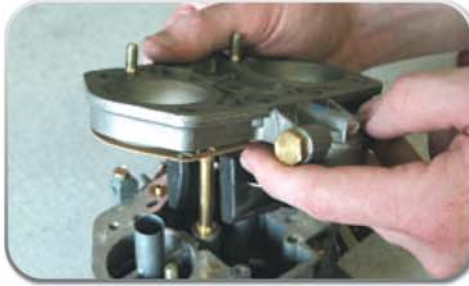
2 - Remove the top off of the carburetor, and remove the gasket.
