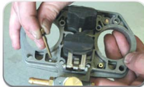
3 - Install the Jet Doctors as shown
