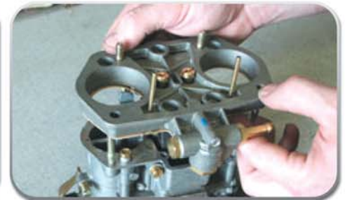
4 - Reinstall the gasket, and then tighten the base to the carburetor.
