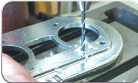
6 - Using the supplied drill bit, drill holes through the air cleaner base.
