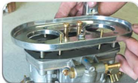
7 - Carefully re-install the A/C base, allowing the Jet Doctors through the holes.
