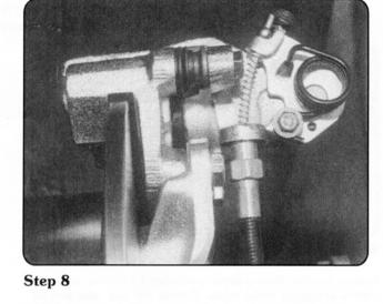
Install the new parking brake cables. Connect the brake lines and bleed the system.
