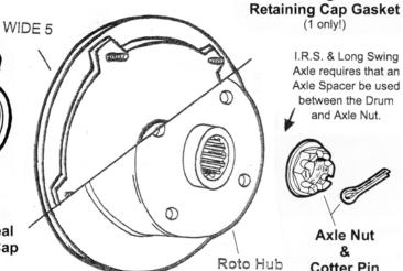
I.R.S. & Long Swing Axle requires that an Axle Spacer be used between the Drum and Axle Nut.
